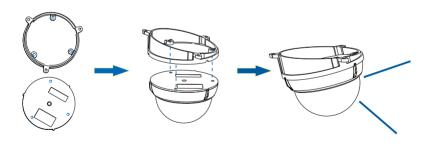
${\it 3. Refer\ to\ the\ steps\ of\ Ceiling\ Mount\ to\ finish\ the\ installation\ of\ slant\ base\ bracket.}$
