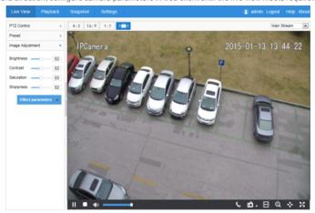
Adjust camera direction and lens angle (Direction: horizontal  $205^\circ$ , vertical  $70^\circ$ ) till the live image in IPCWeb reaches requirements.
