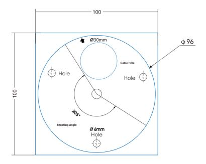
[Notice] This camera can rotate 205° horizontally, so when pasting the installation sticker, the expected surveillance direction should conform to the shooting angle.
